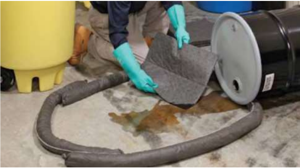
Keep SPILL KITS near work areas with potential spills such as fluid storage.
