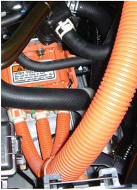
*High-Voltage Cable Connection to Motor*
