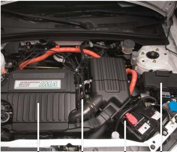
Engine      Motor      12-Volt Battery      Underhood Fuse Box
