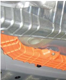
*Electrical shield bolted to undercarriage*
