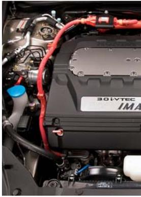
*High-Voltage Cable to Accord AC Compressor*
