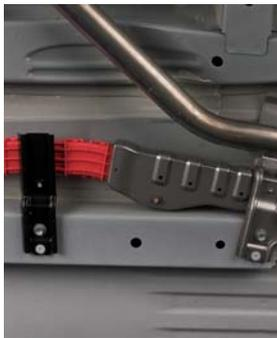
*Thermal shield near hot exhaust*
